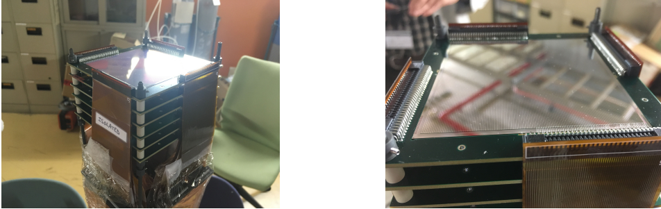
Figure 2.3: AIDA DSSD stack
