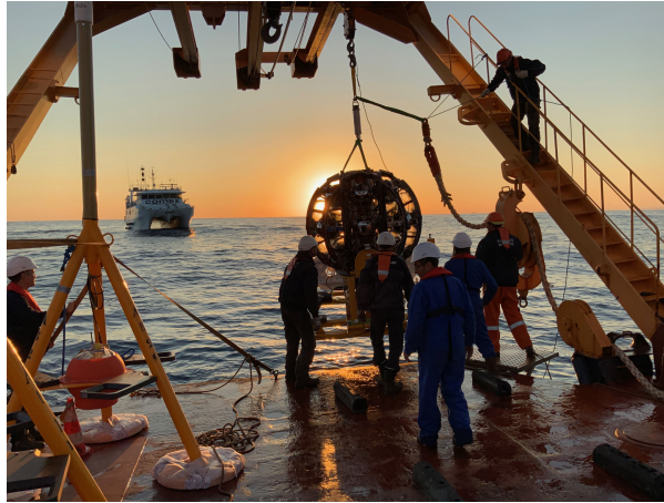
Figure 2.8: A picture of a DU deployment, where the detection unit is furlled into the LOM.
