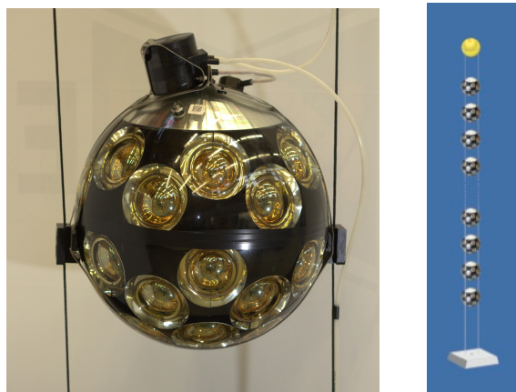
Figure 2.6: On the left, a KM3NeT DOM. On the right, a simplified view of a KM3NeT DU (note that only part of the DOMs are shown, for better visibility of the scheme).
