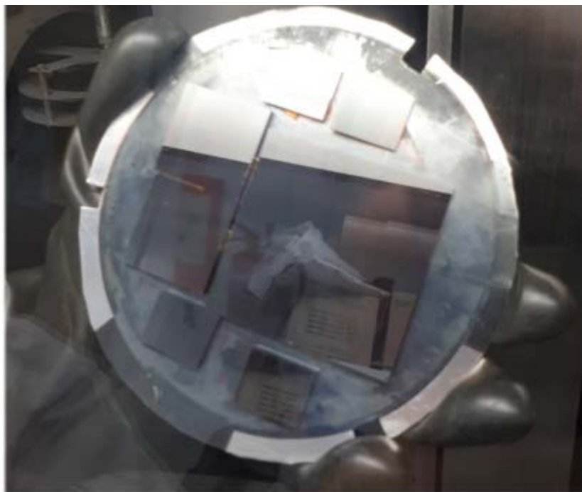
Figure S18: Photos of MAPbI 3 perovskite film. The films have been thermally evaporated in the same batch deposited on substrates of different sizes.
