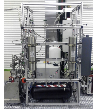
(c) Gas system frame with the getters
