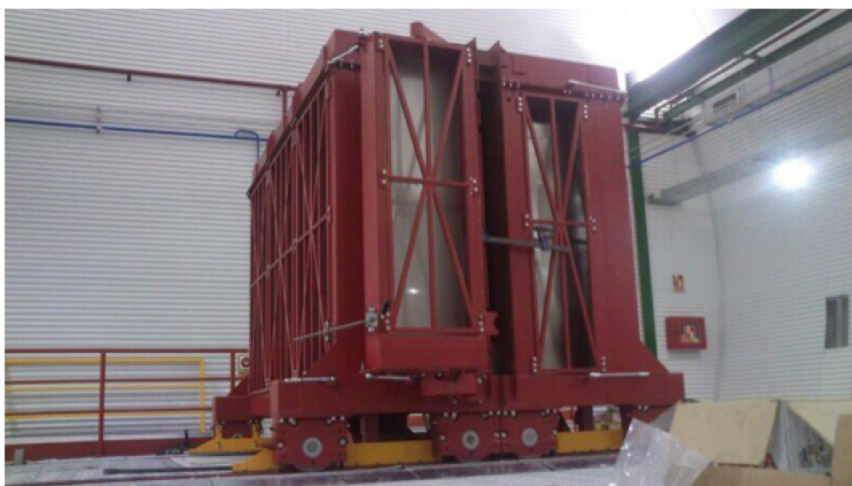
Figure 3.17: Top: Detailed view of the NEXT shielding structure in its open position, with the NEW vessel placed on the anti-seismic platform. Bottom: View of the shielding structure in its closed position during installation.
