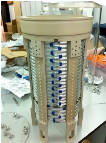
Figure 3.6: Cross-section drawing of the NEXT-DEMO prototype with major parts labelled (top), and image of the field cage standing upright (bottom).
