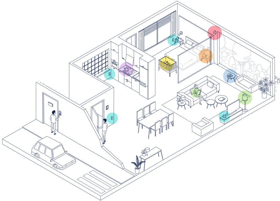
Figure 1.2: Isometric representation of a functional installation of a Visualfy Home. The sky blue color corresponds to the installed devices (detectors and Hub).
