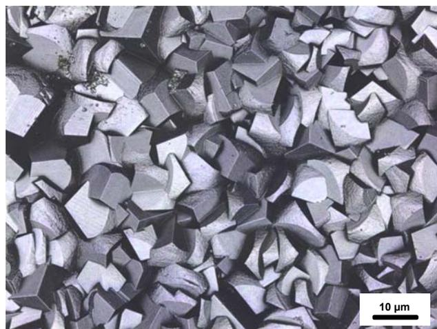
b) confocal image of the scale formed on X-65
