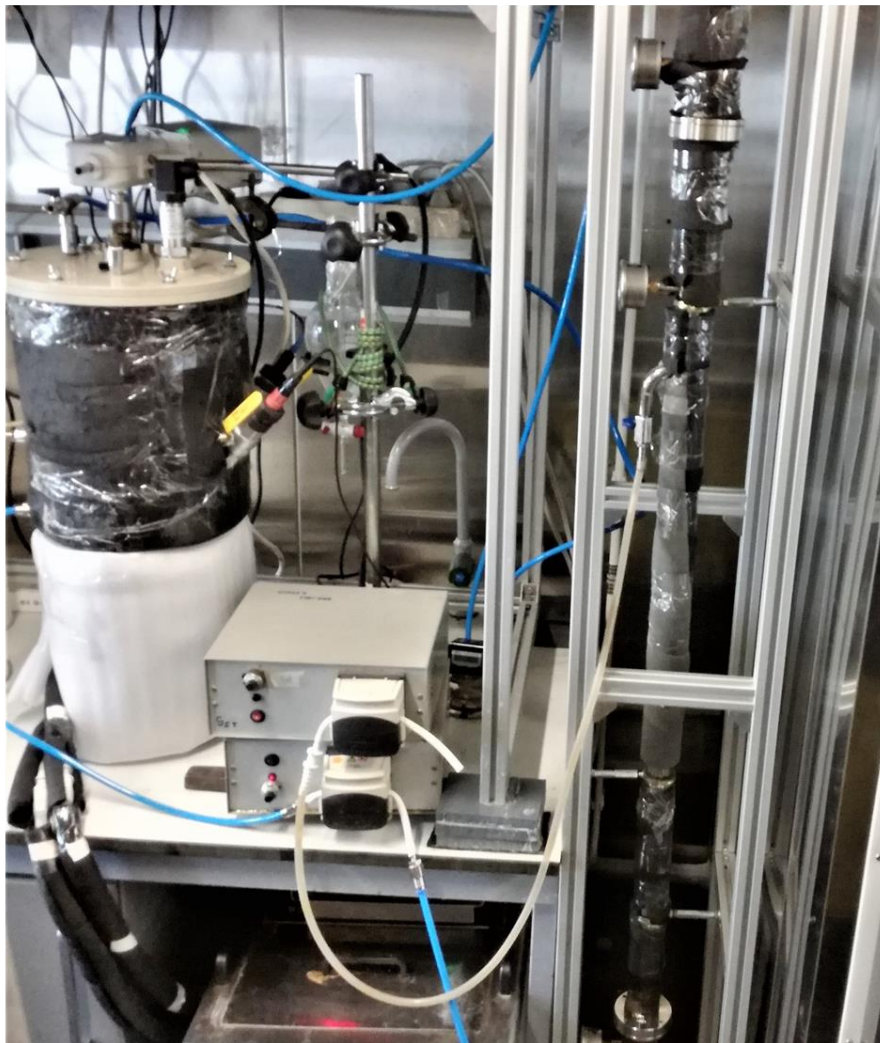
Figure 3.3. Thermophilic lab-scale reactor: layout (a) and experimental set-up (b).
