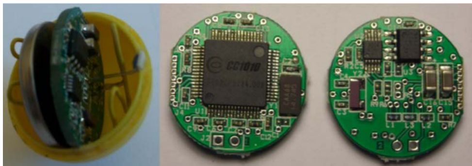
Fig. 13. Autonomous sensor inside its ball-shaped enclosure (left) and layout of the electronic circuit (right) (Martos et al., 2011).
