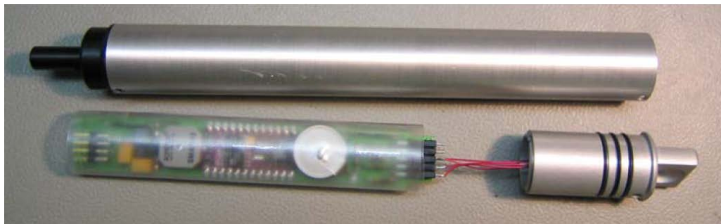
Fig. 10. Data-logger submersible probe to measure pressure and temperature (Rohner et al., 2005).
