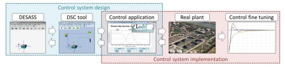
**Figure 5**: Schematic representation of the development procedure for the controllers to be implemented in WWTPs
