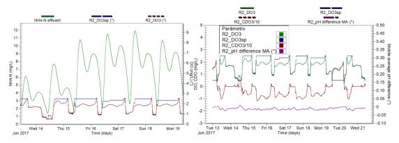
**Figure 6**: Evolution of: (a) DO set point and ammonium concentration in the outlet of the aerobic reactor; (b) inputs to the controller (pH difference, cumulative DO error, DO and DO set point in last aerated chamber); and (c) WWTP effluent nitrogen content within the different scenarios.
