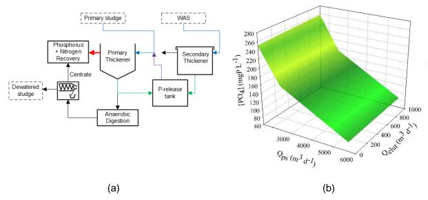
**Figure 3**: (a) Schematic representation of the sludge line configuration simulated (b) concentration of phosphorus in the primary thickener overflow at different operational conditions: primary sludge flow ( $Q_{ps}$ ) and elutriation flow ( $Q_{elut}$ ).
