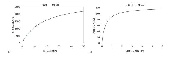
**Figure 4.** OUR values obtained at different substrate concentrations for a) heterotrophic bacteria b) autotrophic bacteria
