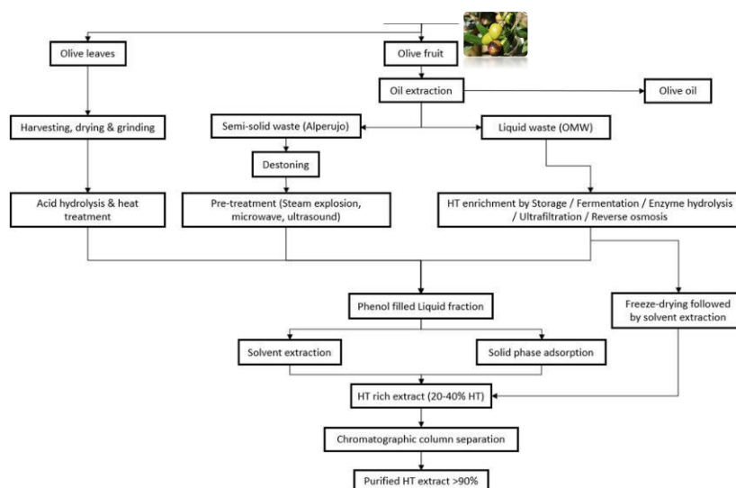
Figure I.19. Flow diagram overview of hydroxytyrosol extraction methods from olive tree derivatives (adapted from Briton et al., 2019)
