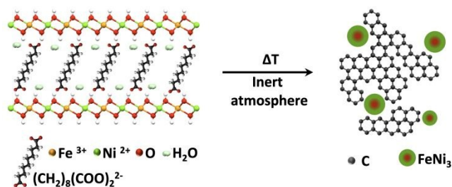
Scheme 1. Thermal decomposition of the hybrid organic–inorganic NiFe-LDH-Seb under an inert atmosphere results in the formation of a nanocomposite consisting of FeNi 3 nanoparticles and a carbon matrix.
