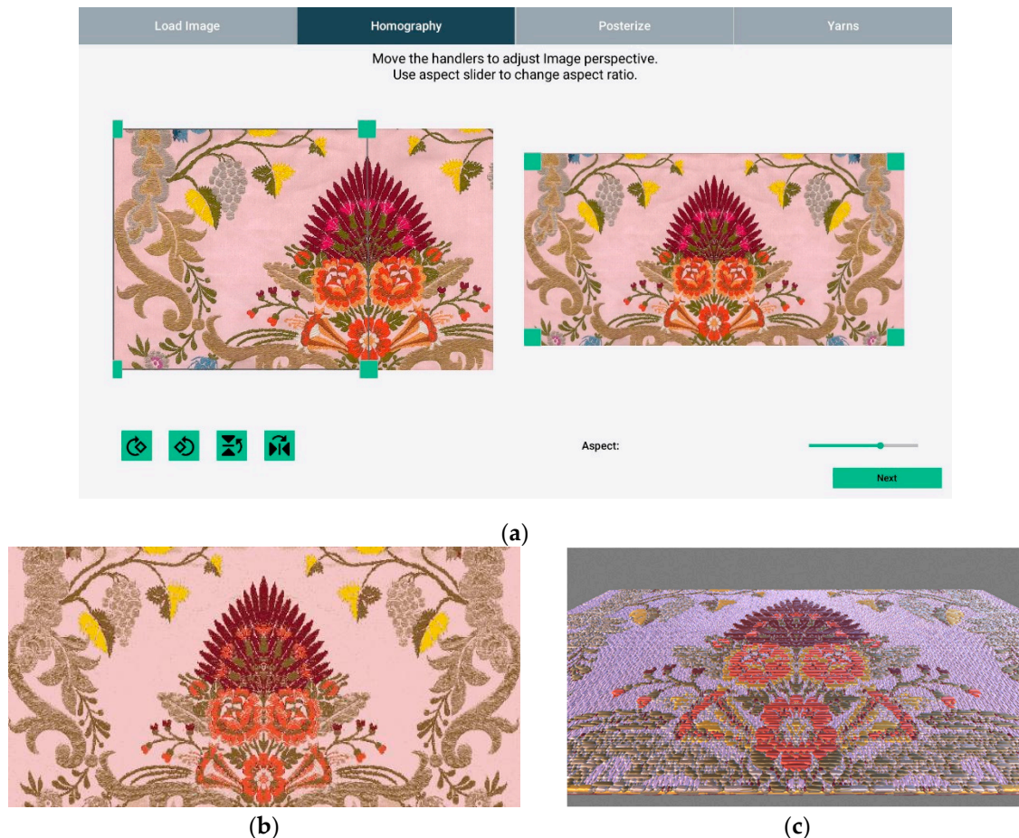
Figure 5. Subtracting the design of a fabric with defect A (only part of the object was pictured), where: (a) Original image and result after applying the symmetry functionality; (b) Reconstructed design; (c) 3D model.
