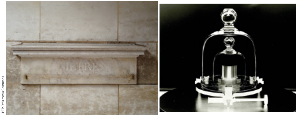
Figure 4. Standards require reference material objects. A) The metre. During the French Revolution, the National Convention had references of the new measurement installed in white marble throughout Paris. The image shows a reference installed on Vaugirard street. B) The kilo. This measurement is another product of the French Revolution. Because its definition as the weight of one litre of water was imprecise, it was redefined using a cylindrical object made of platinum and iridium as a reference. This object is kept at the International Bureau of Weights and Measures in Paris. The kilo has recently been redefined in absolute terms using quantum mechanics. The image shows a replica of the kilogram reference at the U.S. National Institute of Standards and Technology in Gaithersburg, Maryland.
