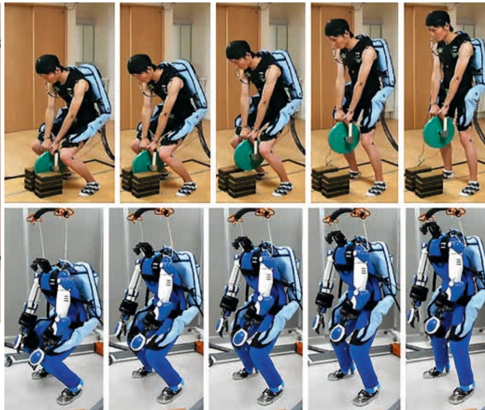
Figure 6. Humanoids can be used to evaluate wearable devices, preventing some of the problems of experimenting on humans, such as the quantitative evaluation of supportive effect as opposed to using subjective questionnaires. In the pictures, evaluation of the pneumatically powered assistive device «muscle suit», which allows a human worker to lift and carry weights greater than they would otherwise be able to, by the humanoid HRP-4.
