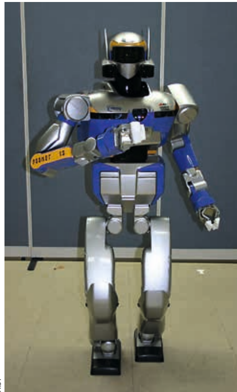
Figure 4. Humanoid robots developed at the National Institute of Advanced Industrial Science and Technology (AIST) in Japan. From left to right: a) HRP-2, b) HRP-3, and c) Cybernetic Human HRP-4C. These robots are intended for uses related to the entertainment industry and their shape is more similar to ours.
