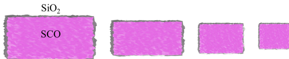
Figure 11. (a) 1D structure of the \text{Fe}(\text{Htrz})_2(\text{trz})(\text{BF}_4) . (b) Scheme of the NPs \text{Fe}(\text{Htrz})_2(\text{trz})(\text{BF}_4)@\text{SiO}_2 synthesized in this thesis with different sizes and morphologies, ranging from nanorods to nanocubes.
