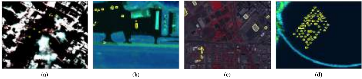
Fig. 1. Images with anomalies (outlined in yellow) in four scenarios. (a) Consequences of the hot spots corresponding to latent fires at the World Trade Center (WTC) in NYC (extension of anomalous pixels represents the 0.23% of the image). (b) Urban area where anomalies are vehicles in Gainesville city (0.52%). (c) Quickbird multispectral images acquired over Denver; the anomalies are roofs in an urbanized area (1.6%). (d) Beach scene where the anomalies are ships captured by the AVIRIS sensor (2.02%) over San Diego, USA.
