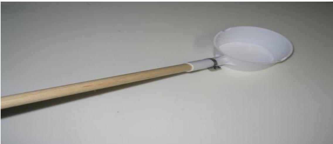
Figura 93: Estructura para la colecta de agua y larvas de mosquito (<https://www.entosupplies.com.au/equipment/field/traps/mosquito-larvae-dipper/>).
