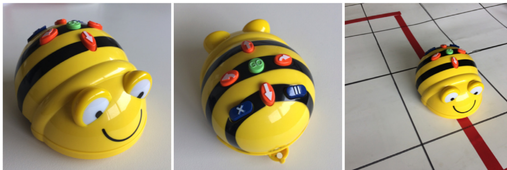
Fig. 1. Bee-bot robot (left). Physical buttons of Bee-bot (centre). 15 cm-grid board for Bee-bot (right).
