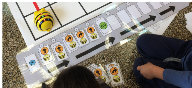
Fig. 2. Cards corresponding to the Bee-bot self-referenced system (top) and physical box to create the Bee-bot program (bottom).
