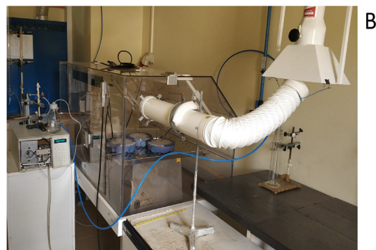
Fig. 1. Scheme (A) and picture (B) of the developed exposition chamber to perform dermal absorption studies. Inset: Picture of glass T-connector to spike clean air with BTEX compounds.
