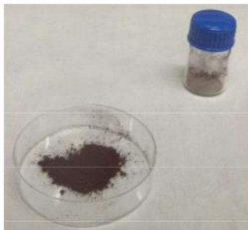
Figure S3. UV-Vis optical absorption for powders obtained by mechanochemical and melting techniques. A photograph of as-prepared perovskite from mechanochemical synthesis is shown as reference.
