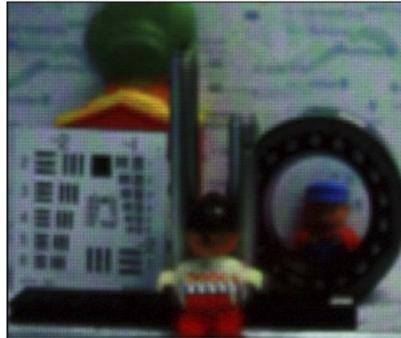
**Fig. 3.** Displayed 3D image as seen by a monocular observer (a photography camera in our experiment) placed in front of the lightfield monitor. In [Visualization 1](#) we can observe the parallax of such image.
