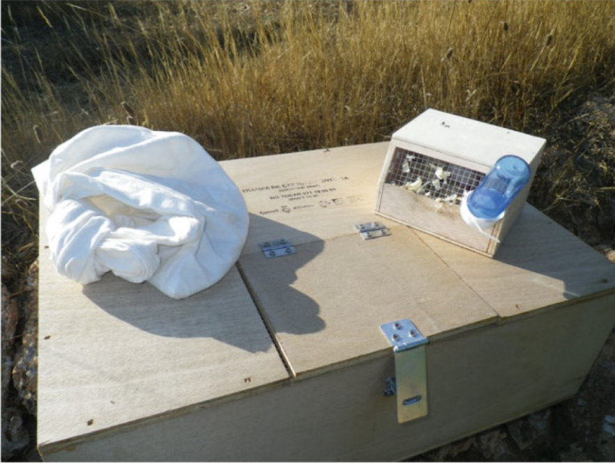
Fig. 5.5 Wooden box trap for capturing snakes on Ibiza Island. Note the access hatch on the top, a funnel in the lateral, and the small cage for restraining the lab mouse within the snake trap. Photo by E. Ayllón
