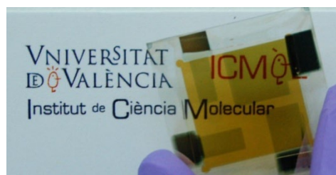
Fig. 5 Photograph of the semitransparent solar cell having a 100 nm perovskite layer resulting in an AVT ~ 30% and a PCE of 6.4 %.
