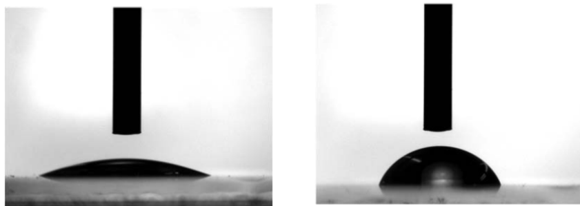
Figure S3. Contact angle measurements of a MoO 3 thin film (left) and a MoO 3 thin film with 2 nm of TPBi on top (right).
