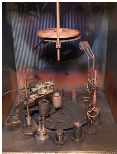
Figure 9: Basic schematic of the evaporation chamber and real picture of a similar chamber.
