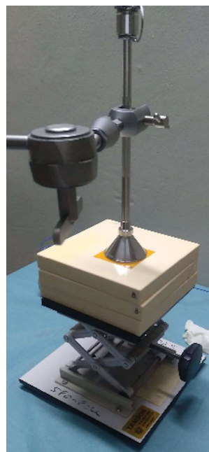
Fig. 2. Measurements with the Xoft 50 mm diameter skin applicator for calibration of XR-RV3 radiochromic films.
