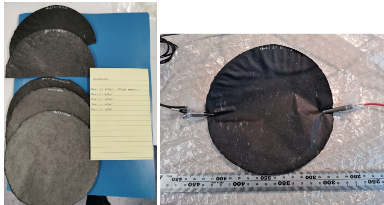
Figure 6.3: Left: 16 cm diameter Smart Paper samples with different concentrations of CNTs. Right: Smart Paper sample under measurement
