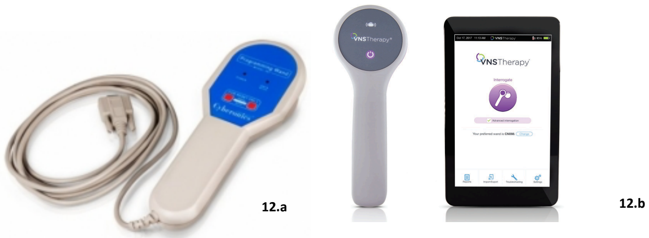
Figure 12: 12.a): VNS telemetric wand and the cable (old model-a-). 12.b): Programming wand (M2000) and programmer (M3000) (Models Aspire106SR and SenTiva). (Obtained from: 12.a) www.medicaexpo.com/prod/cyberonics/product-84639-544485.html ; 12.b) www.medgadget.com/2017/10/livanovas-new-sentiva-neurostimulator-epilepsy-fda-approved.html ).
