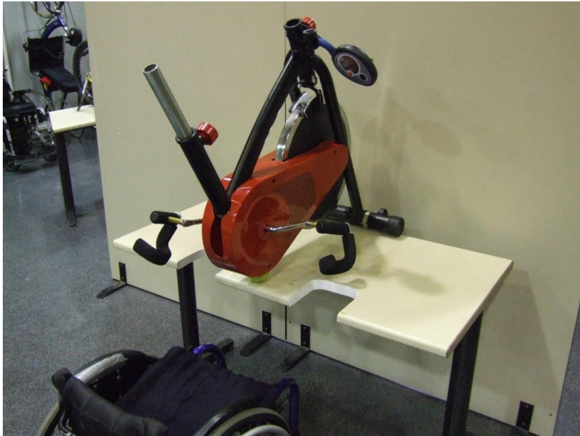
Figure 1. Special adjustable hand grips designed for persons without grip ability and mounted onto the custom designed armcrank ergometer.
