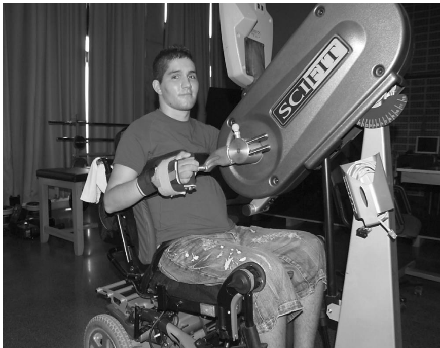
Figure 3. Fully adjustable adapted ergometer used to measure the ACE power output.
