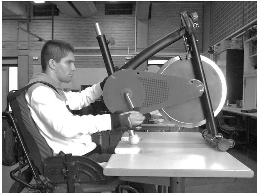
Figure 2. Adjustable-height armcrank ergometer as used for training.
