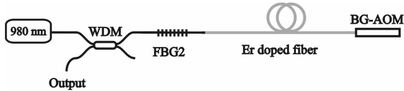
Fig. 4. The Q-switched all-fiber laser arrangement.
