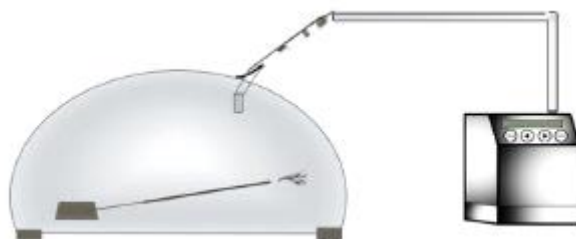
Figure A11. Design of the system for collecting vapor from incense sticks or cones.
