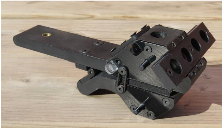
Figure 4-5 Picture of the FluoWat leaf clip in its final design.
