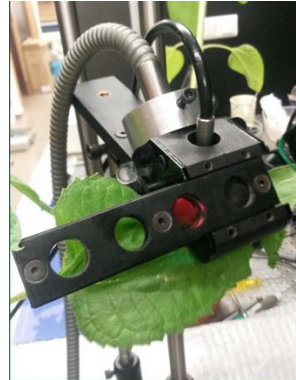
Figure 4-7 Dark adapting a leaf with a PAM fibre attached at the back port
