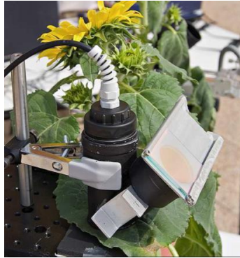
Figure 4-3 First evolution introducing novel characteristics, such as removable filter and sun finder, but not yet including transmittance.
