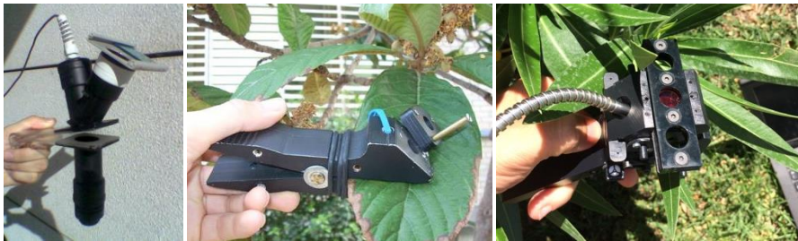
Figure 4-4 Pictures of some early prototypes (left, centre) of the FluoWat leaf clip and the final design (right).
