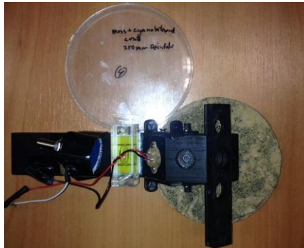
Figure 5-10 The FluoWat leaf clip, with the bottom part removed to measure on thick solid samples. The LED in the back port was not used in this experiment.
