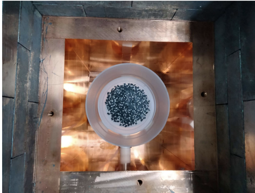
Figure 9.1.: Example of a sample analyzed at the Radiopurity Service of the LSC for NEXT. In this case, the screened items are capacitors to be used in the PMT bases of NEXT-100, and the specific detector is the Anayet .
