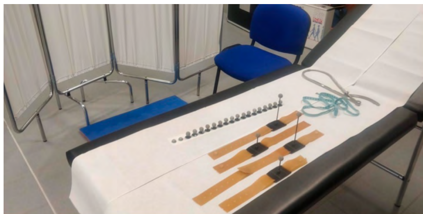
Figure 42. Markers and measuring instruments for gait analysis using the optoelectronic system.
