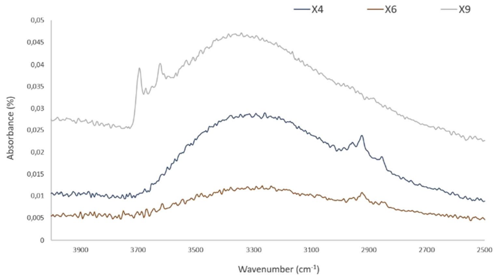
Fig. 9 FTIR-ATR spectra of samples X4, X6 and X9. In samples X4 and X6, a weak peak at \sim 2919\text{ cm}^{-1} of an organic fraction is observed. The X9 sample spectra show two peaks at 3688 and 3616\text{ cm}^{-1} typical of OH group
