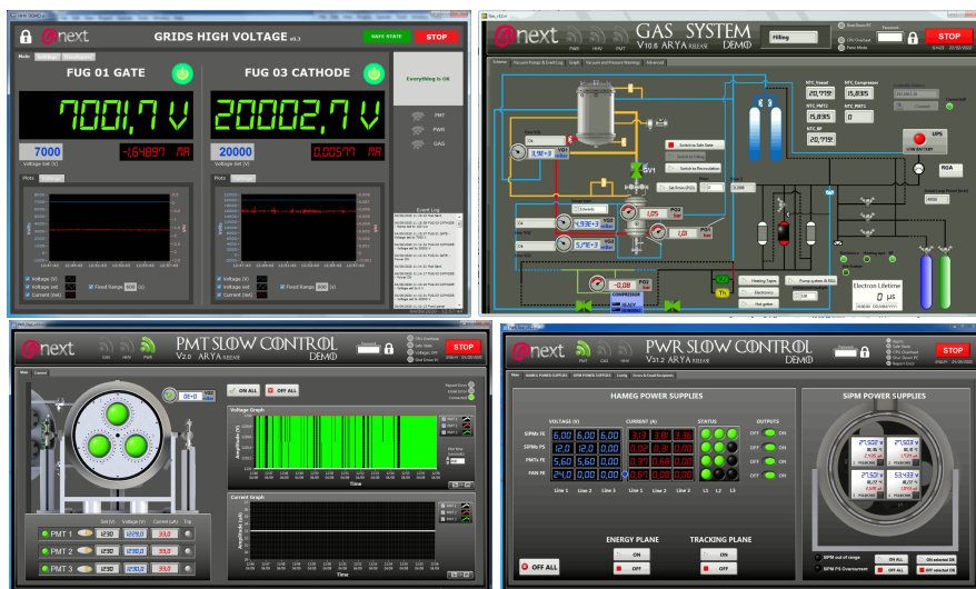
Figure 5.17. Main window of the slow control programs managing the high voltage (top left), the gas system (top right), the PMTs voltages (bottom left) and the SiPMs voltages and sensors front end electronics (bottom right).
