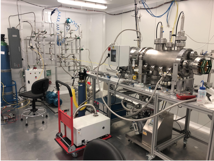
Figure 5.1. General view of the detector NEXT-DEMO++ inside the clean room. The gas system can be seen on the background. Below the table supporting the detector are located the high voltage power supplies and the turbomolecular pump.
