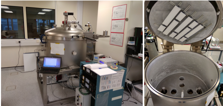
Figure 5.8. Evaporator during operation (left) and installation of the teflon panels in the rotating disk of the evaporator prior to operation (right). The evaporator was used through the courtesy of the neutrino group of the University of Manchester.
