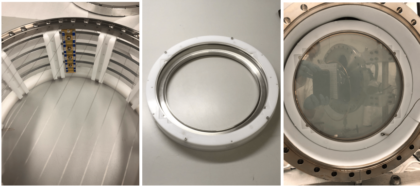
Figure 5.5. Cathode frame mounted on the buffer section of the field cage (left). The tensioned stainless steel wires can also be seen. Mesh frame embedded in its HDPE support (center). The mesh, being too thin, can not be seen on the picture. Anode plate housed in its HDPE support (right). On that picture the anode plate is mounted on the field cage which is inside the pressure vessel.
