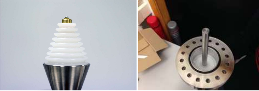
Figure 5.7. High voltage feedthroughs operated in NEXT-White. The one connected to the cathode is on the left and the one connected to the gate is on the right. Those used for NEXT-DEMO++ were built following the exact same design.
