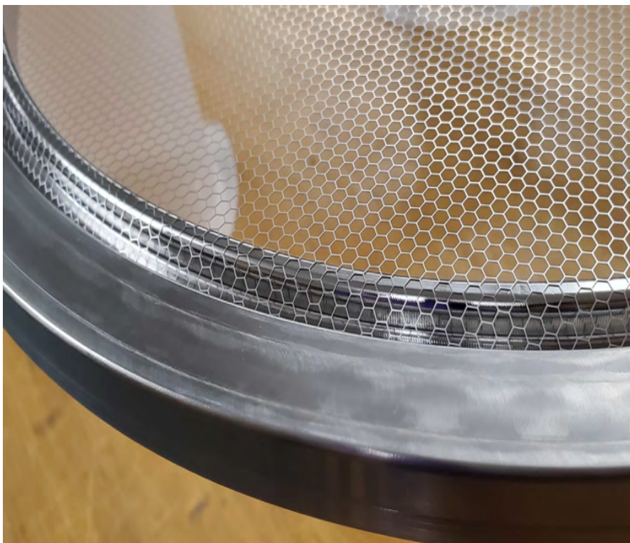
Figure 3.16. Picture of the tensioned cathode for NEXT-100. The hexagonal pattern of the grid can be seen.
