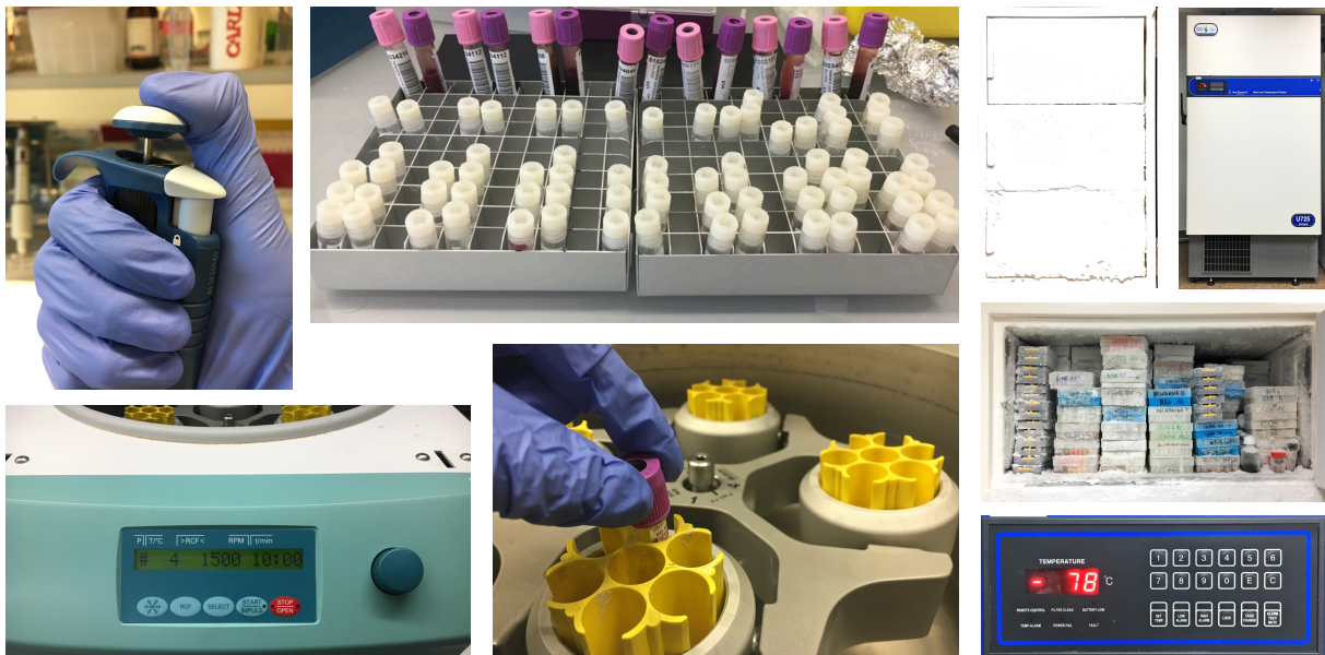
Figure 16. Samples from the hospital are centrifuged, aliquoted and frozen until the experiments.
