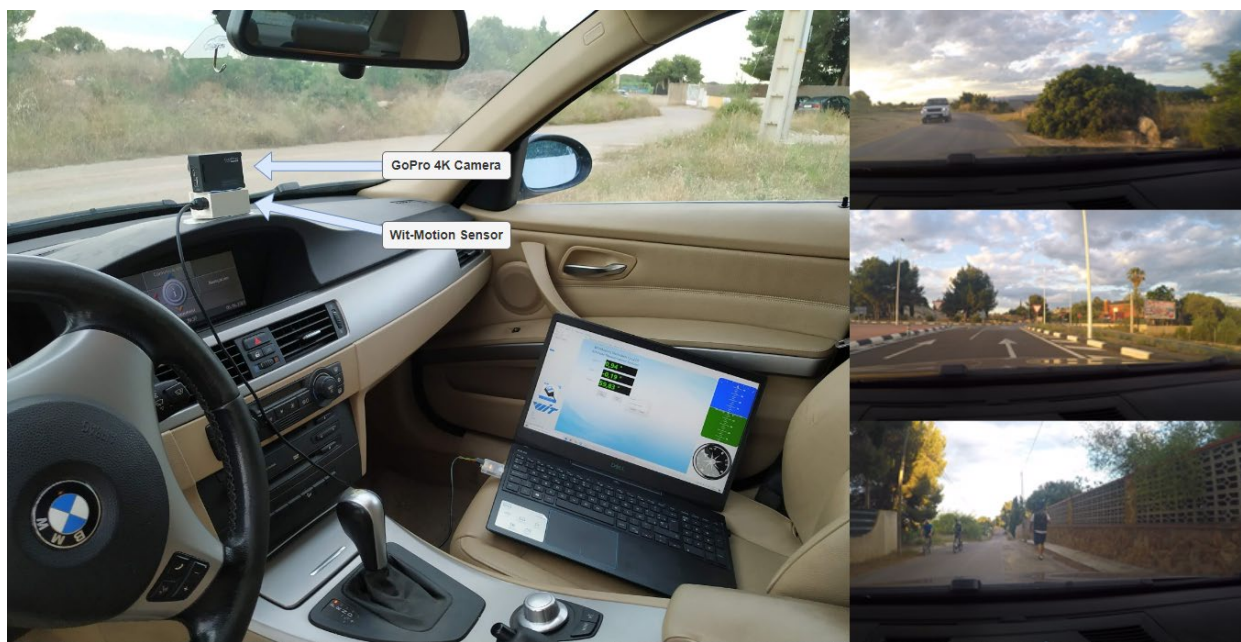
Figure 3. Sensor, camera and laptop installation for real-time sample collection.
