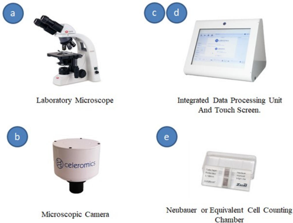
Figure 30: Elements of the improved cell counting method.
