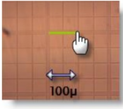
Figure 31 : The process of system calibration is performed by selecting a segment of 100 \mu\text{m} on the screen
