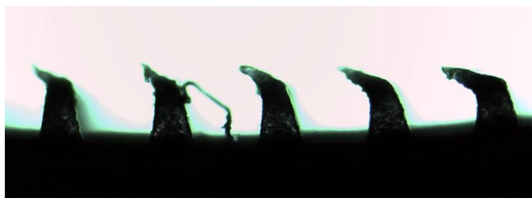
Figure 6.21. F9 deformed-needles after compression mechanical test.
