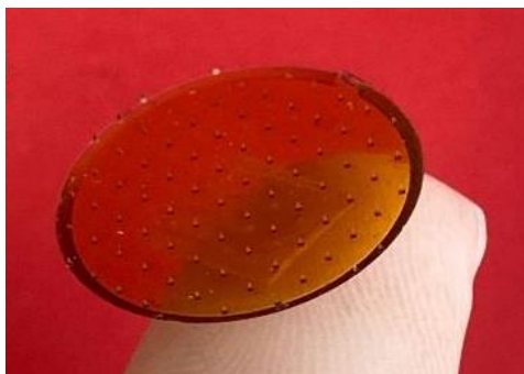
Figure 7.6. Solid microneedles used to create micro-pores in the porcine skin.
