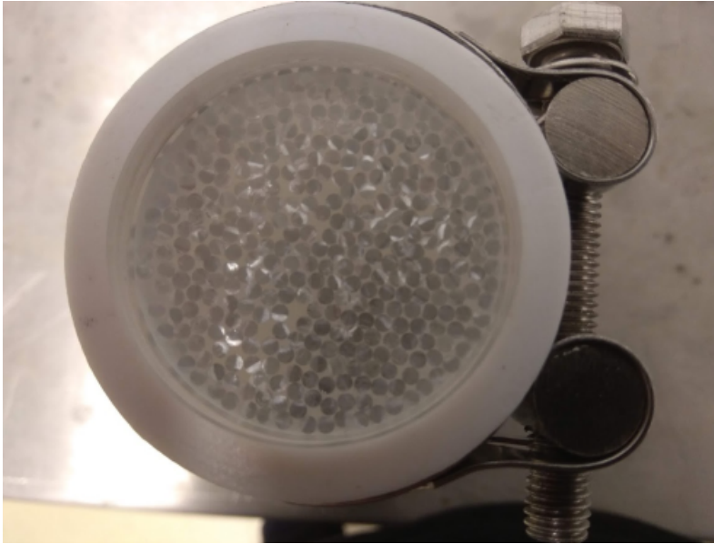
Figure 5.10 – PTFE vessel and fibre bundle used in TRITIUM-Aveiro prototype.
