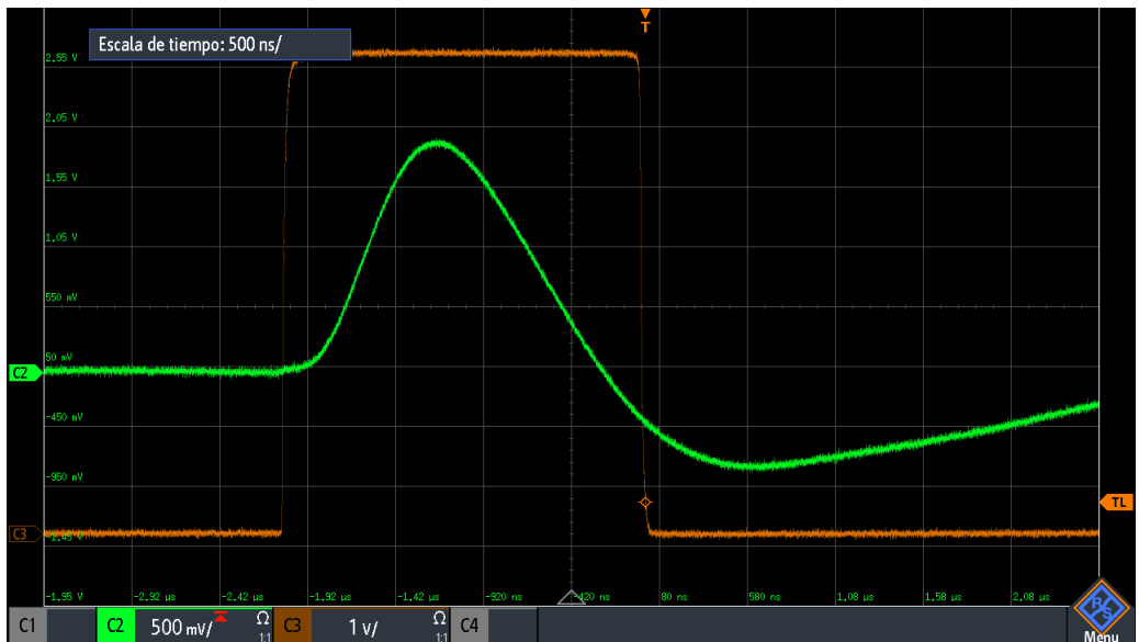
Figure 3.17 – Amplified signal and logic gate (input signals of the MCA).
