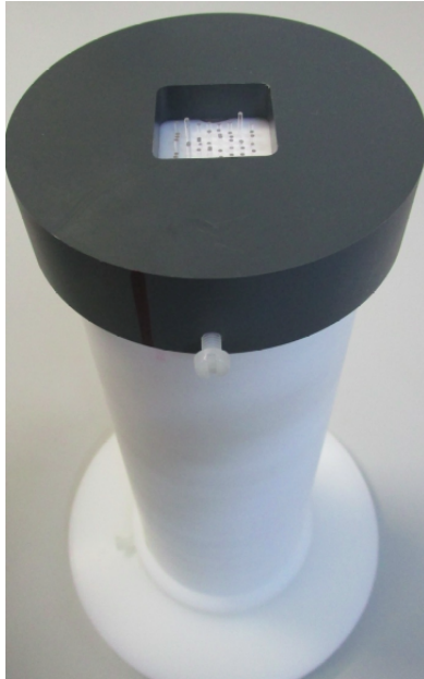
Figure 5.7 – Picture of TRITIUM-IFIC-1. The photosensor lodging is shown.
