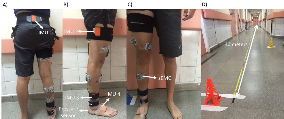
FIGURE 1 | Sensors locations and 30 m used corridor. (A) Back view. (B) Lateral view. (C) Frontal view. (D) Walking assessment corridor. Surface electromyography (sEMG), inertial sensor positioned in pelvis (IMU 1), inertial sensor positioned in lateral face of thigh (IMU 2), inertial sensor positioned lateral face of the shank (IMU 3), and inertial sensor positioned in midfoot (IMU 4).
