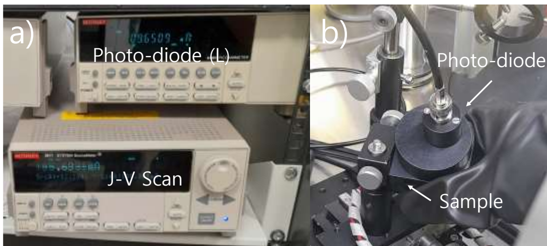
Figure 3.7. a. Keithley setup for device characterization. b. Measurement configuration employing photodiode to evaluate luminance.
