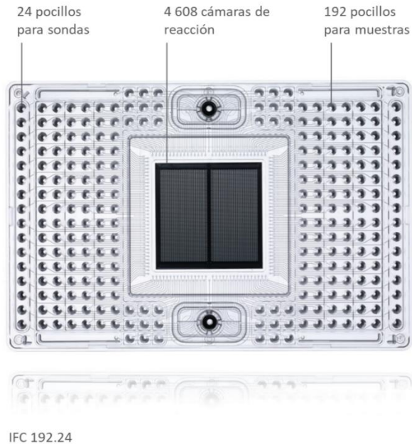
Figura 5. 192.24 Dynamic Array™ integrated fluidic circuit (IFC). (Fuente: www.fluidigm.com )
