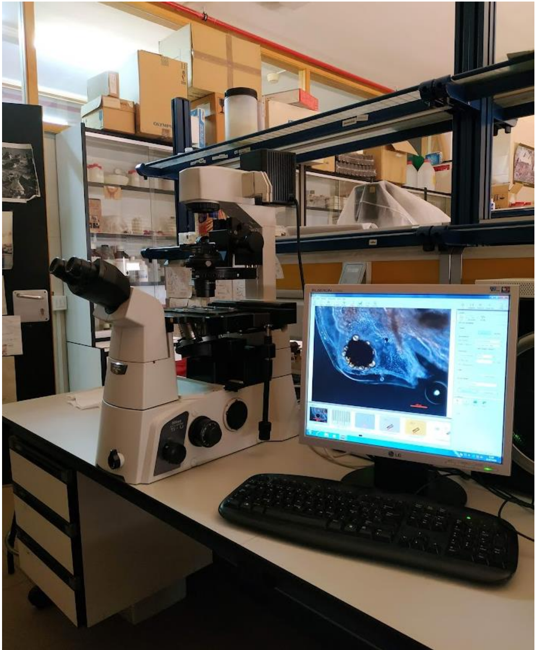
Inverted microscopy for species identification and counting Laboratory of Limnology, Department of Microbiology and Ecology Valencia University, 2022.
