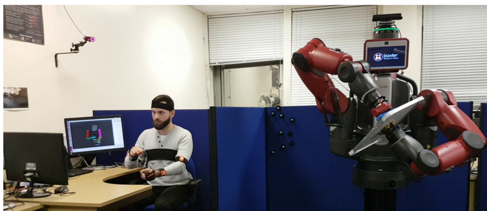
(a) Both arms with inertial motion capture teleoperation.
