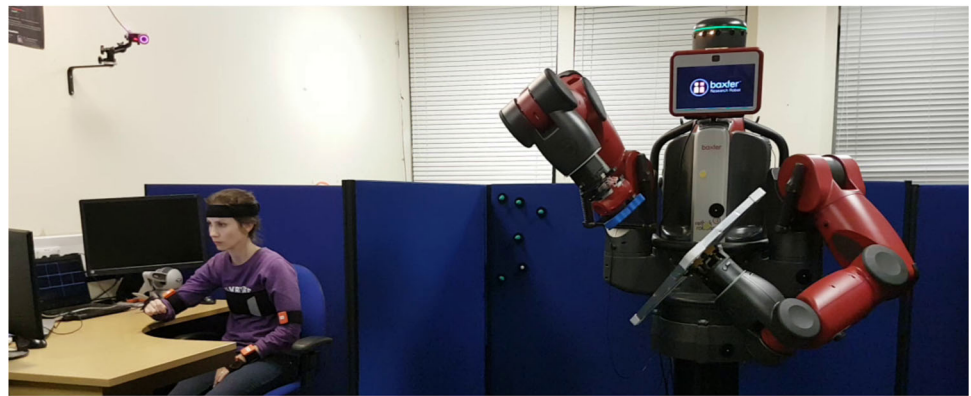
(b) Right arm teleoperation with motion capture system
