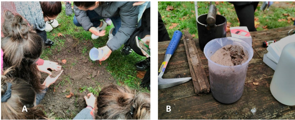
Figure 1. Measurements during the TLS: (a) Students taking measurements on the soil in the OLG, namely, sampling soil to add hydrogen peroxide to get a measure of the organic matter content. (b) Some of the instruments needed, and reaction of the soil in contact with hydrogen peroxide (intense).
