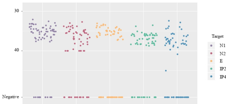
Fig. 2. Distribution of cycle threshold values for N1, N2, E, IP2 and IP4 genomic targets of SARS-CoV-2 detected in wastewater samples (n = 34 samples).
