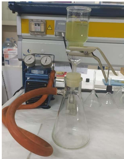
Figure 5.2: Assembly employed for water filtration.
