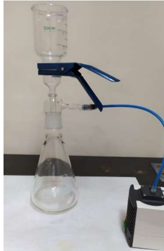
Figure 4.1: Set up to filter the water.
