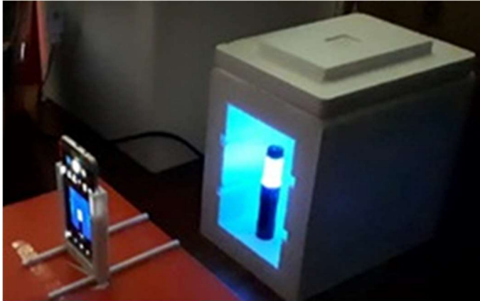
Figure 8.2: Set-up to take the fluorescence measure by smartphone.
