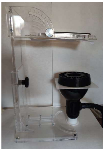
Figure 9.3: Methacrylate support to take the photograph.
