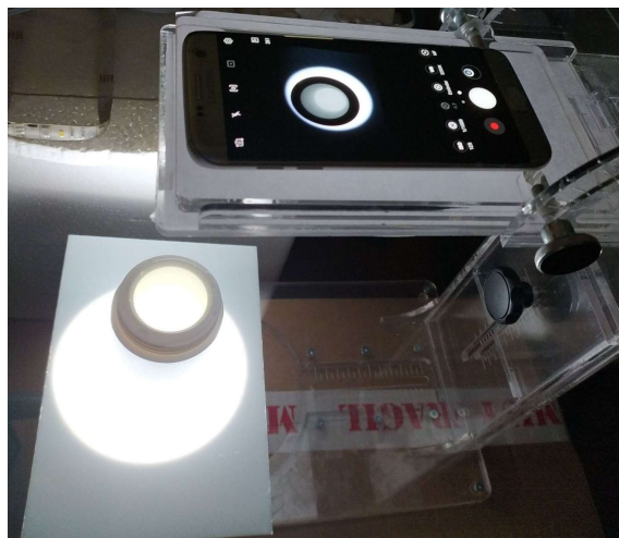
Figure 5.1: Assembly employed to take photos of the water column by Smartphone.
