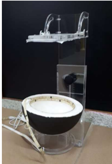
Figure 1.2: Methacrylate support employed to obtain the images by the smartphone devices.
