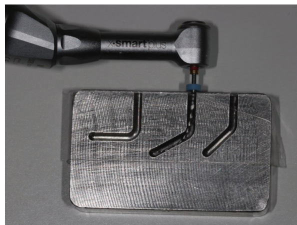
Fig. 2: Clamping mechanism of the handpiece for the X-Smart Plus endo motor.
