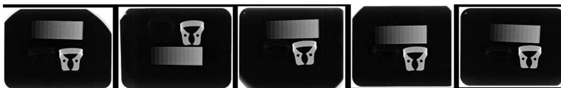
Fig. 1: Illustration of the radiographs of the polymer and conventional metal clamps together with the aluminum scale.
